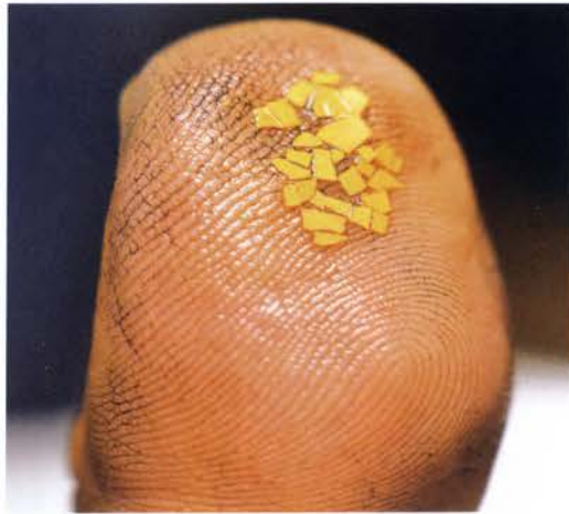
■ Fig. 6a & 6b. The process of finish polishing ( shiage-tōgi ) by moving finger stones over the blade.
